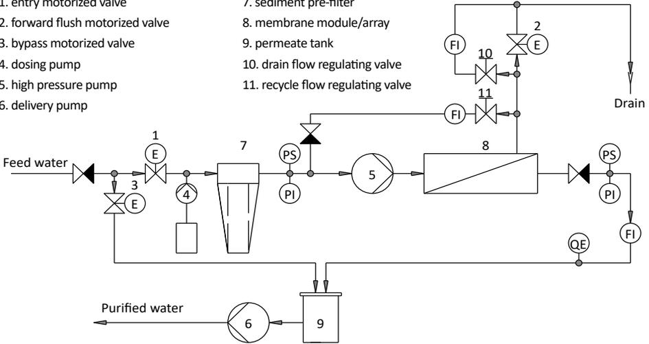
Figure 1. Reverse osmosis system with raw water blending
