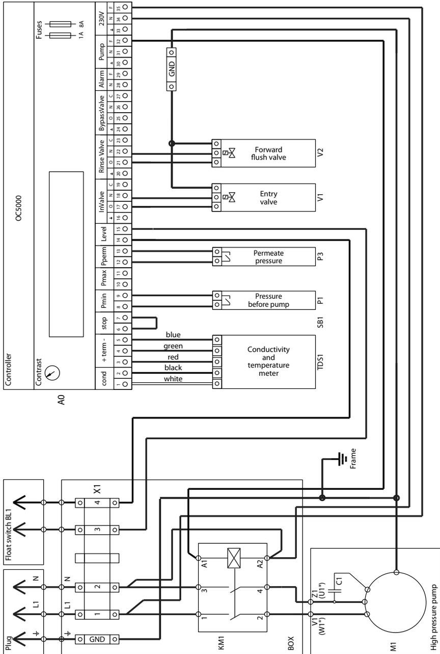
Figure 1. OC5000 wiring diagram for MO-6500, MO-12000 and MO-24000 (230 V)
