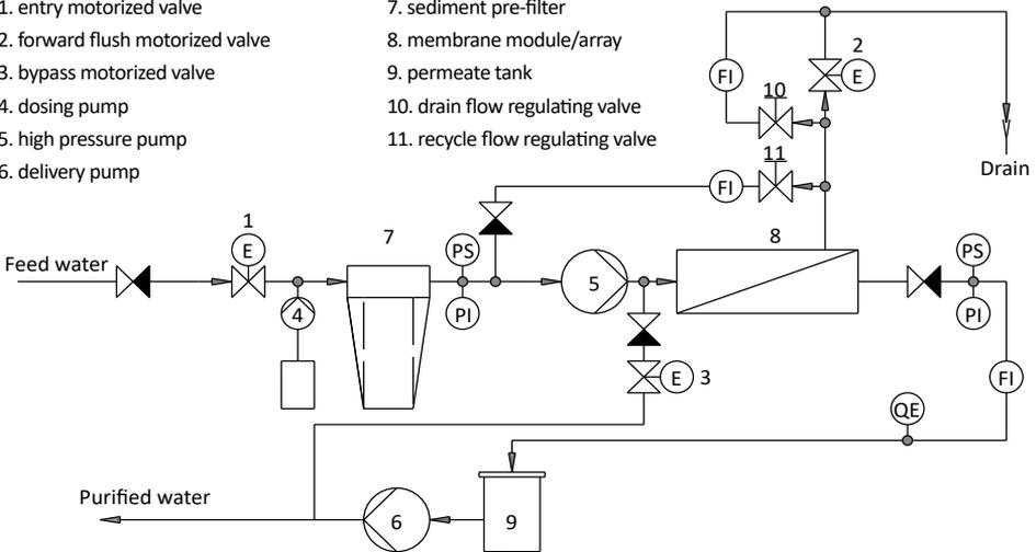
Figure 2. Reverse osmosis system with permeate rinsing
